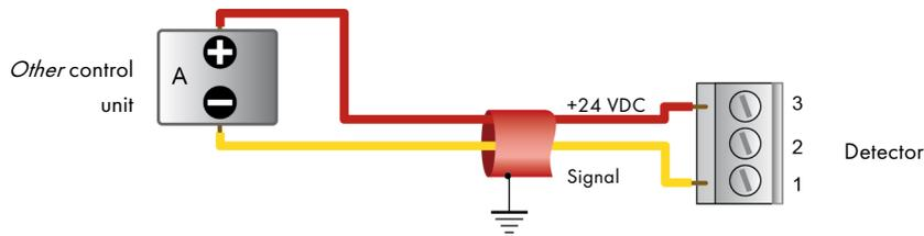
**Figure 8:** Connection of a 2-wire 4-20mA sensor to a non-TELEDYNE OLDHAM SIMTRONICS control unit.
