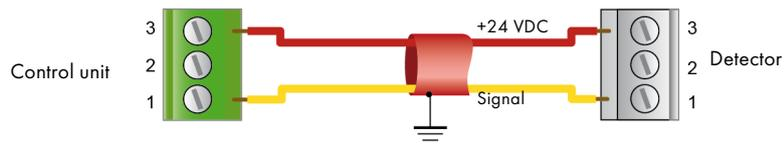
Figure 6: connection of a 2-wire sensor to an TELEDYNE OLDHAM SIMTRONICS control unit.
