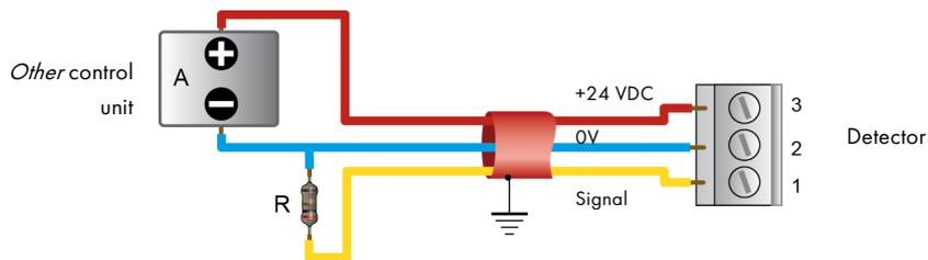
Figure 7: Connection of a 3-wire CTX300 sensor to a non-TELEDYNE OLDHAM SIMTRONICS control unit.
