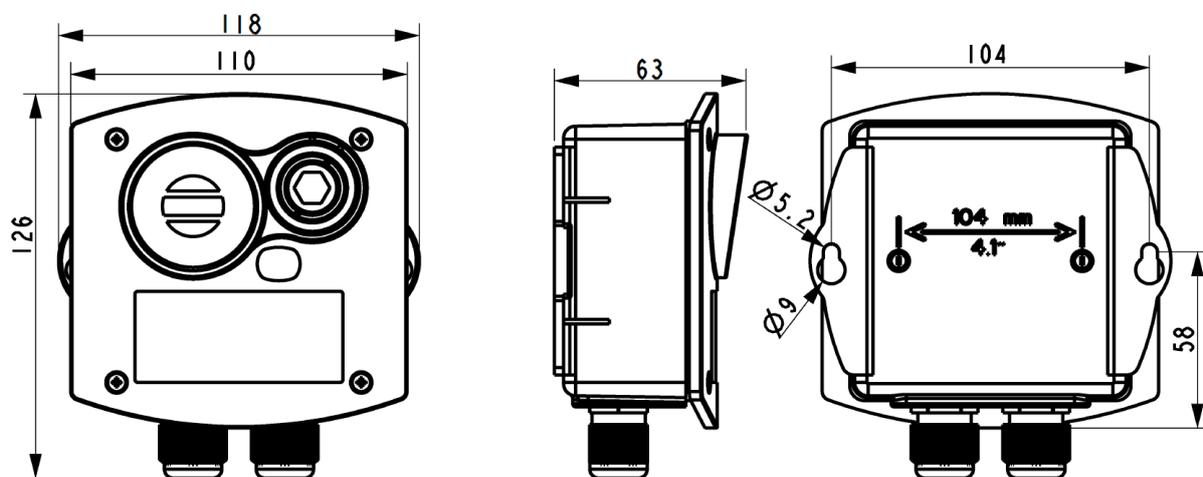
Drill two holes 104 mm apart on the base to mount the units.
