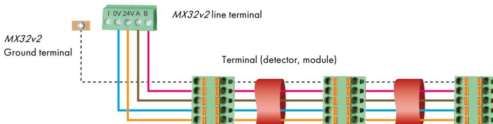
Figure 11: Connection of the modules on a line
