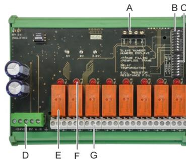
Figure 15: 8 relay module
