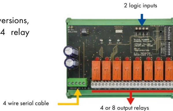
Figure 14: 8 relay module
