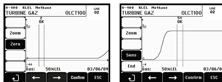
Figure 39: Adjustment of zero (left) and sensitivity (right)
