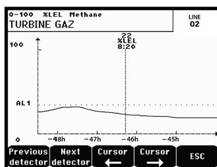
Figure 36: Example of a curve display screen
