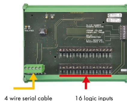
**Figure 16: 16 Logic Input Module**
