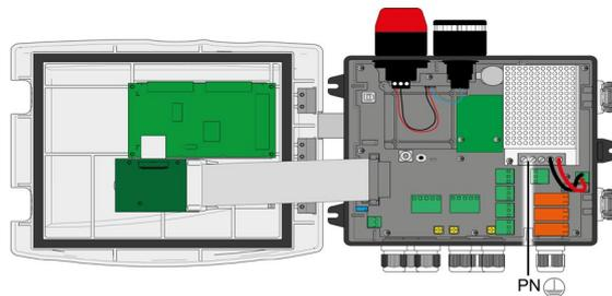
Figure 22: Connection of the main power supply
