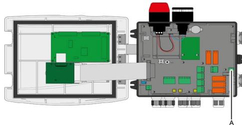
Figure 23: Connection of 24Vdc external power supply (A)
