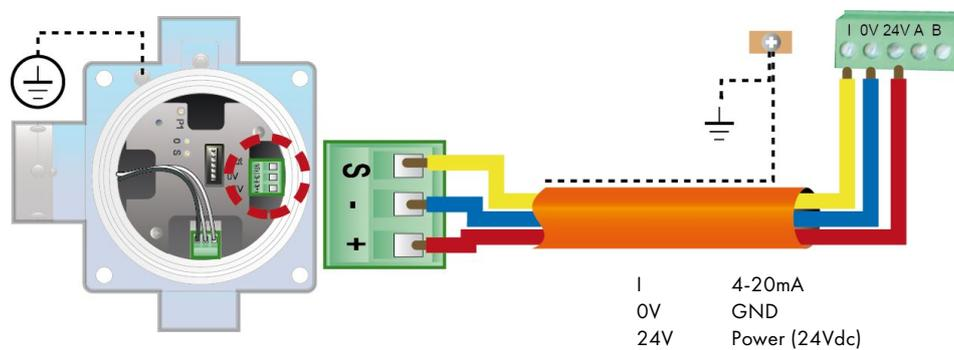
Figure 25: 4-20mA detector connected to an analog line
