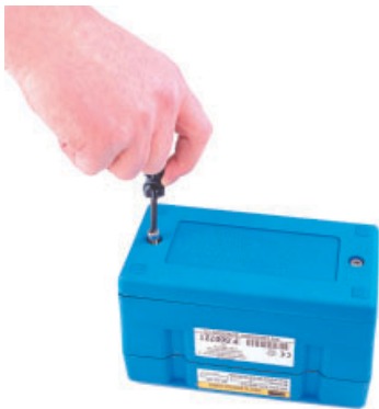
Fig. 5-5 Loosen Instrument Base Screws
