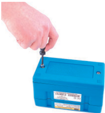
Fig. 5-3 Loosen Instrument Base Screws
