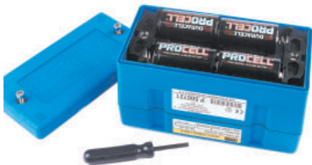
Fig. 5-6 Remove Battery Cover
